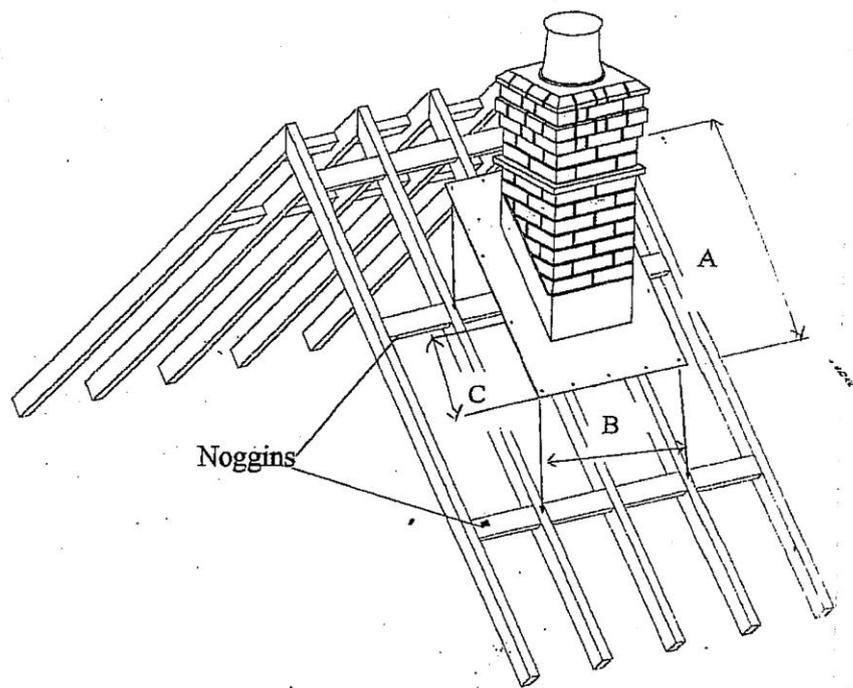
NB *Litestack* Chimneys should be fitted after the rafters are secured in place but before the roof is felted or the laths are fitted.
